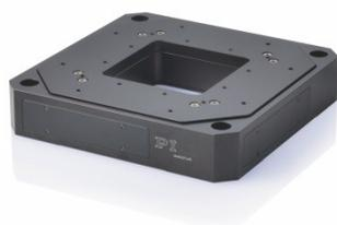
The piezo-based scanning stage is essential for sample positioning. It is designed for working distances of 100 or 200 µm in the axes of the scanning plane and 30 µm in the Z axis. It allows a position resolution of better than 2 nm. Capacitive sensors and digital electronics provide maximum stability.
