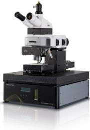
The modular microscopy systems from WITec make it possible to combine a confocal Raman microscope with atomic force microscopy (AFM).
